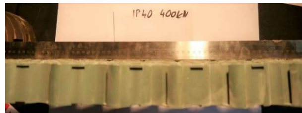
Photo.6. IP 40 after the test at 400kN
