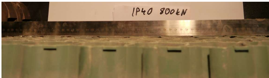
Photo.7. IP 40 after the test at 800kN
